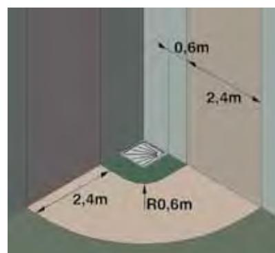
Safety area in accordance with DIN VDE 100 (Part.701) for installing a dryer, distance in metres.
